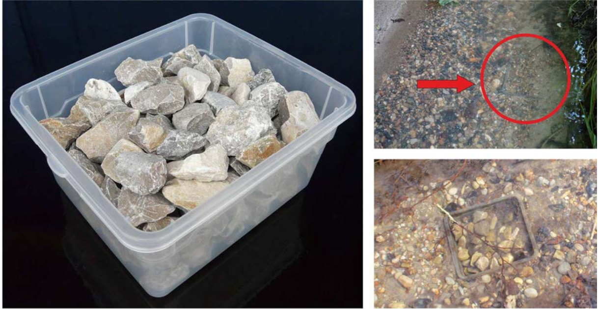
Figure 2.5 Sediment trap filled with gravel in grain sizes of 22–32 mm (left) and sediment traps buried in the river bed at the end of the exposure period (right).
